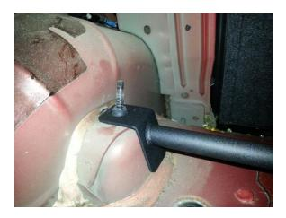
4. Reinstall the rubber bushing and metal top, and then retighten the strut tower nut to factory spec.
