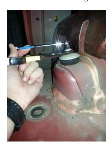
3. Remove the metal top and rubber bushing and install the brace.
